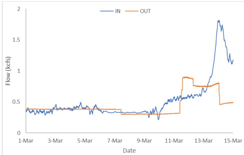
**Figure 36. Hourly Flows Inflow vs. Outflow (RO) (Fall Creek Tailrace)**
